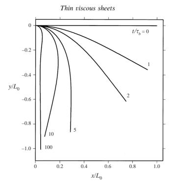
FIGURE 7. Deformation under gravity of an initially horizontal 'viscous beam' with its left end clamped and its right end free. The beam's initial length and thickness are  $L_0$  and  $H_0 = 0.05L_0$ , respectively, and the bending time scale  $\tau_b$  is defined by (7.8).
