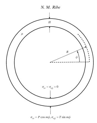
FIGURE 2. Model problem for scaling analysis and evaluation of the accuracy of the thin-sheet equations. A cylindrical annulus with mean radius R, thickness H, and viscosity  $\mu$  is deformed by a normal stress  $\sigma_{rr} = P \cos m\phi$  and a tangential stress  $\sigma_{r\phi} = T \sin m\phi$  applied to its outer surface r = R + H/2. The sheet's inner surface is stress-free.
