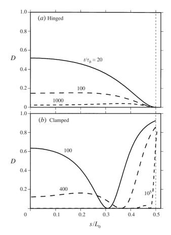
FIGURE 4. Local dissipation ratio D at various times for a blown film with  $\epsilon = 0.005$  and either hinged (a) or clamped (b) ends. Only the portion  $s \ge 0$  of the sheet is shown, and the fixed end is at the right. The curve for a clamped sheet at  $t/\tau_b = 10^5$  extends beyond  $s/L_0 = 0.5$  by an amount equal to the total stretching of the sheet up to that time. Bending time scale  $\tau_b$  is defined by (7.4).
