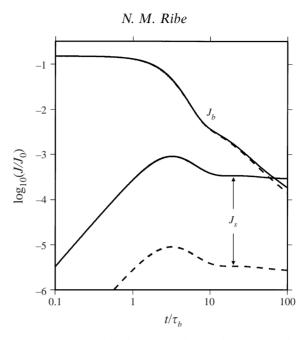
FIGURE 8. Total dissipation rates  $J_b$  and  $J_s$  due to bending and stretching, for a viscous beam with  $\epsilon = 0.05$  (figure 7) (solid lines), and  $\epsilon = 0.005$  (dashed lines). The bending time scale  $\tau_b$  is defined by (7.8), and  $J_0 = \epsilon^3 \mu L_0^2 / \tau_b^2$ .
