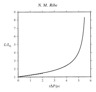
FIGURE 6. Length as a function of time of the blown films whose shapes are shown in figure 5.
