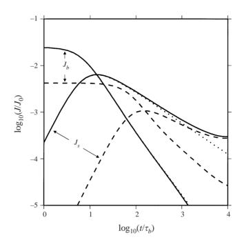
FIGURE 3. Total dissipation rates  $J_b$  and  $J_s$  due to bending and stretching, respectively, as functions of time for blown films with initial length  $L_0$  and thickness  $H_0 \equiv \epsilon L_0$ . Solid lines:  $\epsilon = 0.05$ , hinged ends. Dashed lines:  $\epsilon = 0.05$ , clamped ends. Dotted lines:  $\epsilon = 0.005$ , hinged ends. Bending time scale  $\tau_b$  is defined by (7.4), and  $J_0 = \epsilon^3 \mu L_0^2 / \tau_b^2$ .
