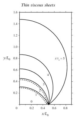
FIGURE 5. Shape of a blown film with  $\epsilon = 0.05$  and either hinged (solid lines) or clamped (dashed lines) ends. Only half (s > 0) of the sheet is shown. Evolution of the clamped sheet was not followed beyond  $t/\tau_s \sim 2$  because the bending boundary layers become too thin to resolve numerically. Stretching time scale  $\tau_s$  is defined by (7.5).
