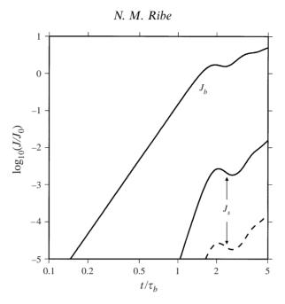
FIGURE 10. Total dissipation rates  $J_b$  and  $J_s$  due to bending and stretching for horizontally extruded sheets with  $\epsilon = 0.05$  (solid lines) and  $\epsilon = 0.005$  (dashed lines). Solid and dashed lines for bending coincide.
